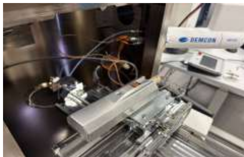
Fig.1: JT microcooler device on a Zeiss GeminiSEM 460
