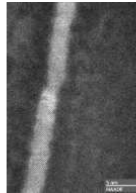
Fig. 2: Multiple shearing of fibrous VC nanoprecipitates.
