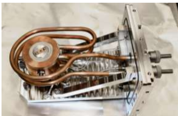
Fig. 1: TM_{110} dual mode deflection cavity.
