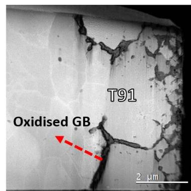
Fig. 2: STEM HAADF view of the TEM lift out foil of oxidising environment corroded sample.
