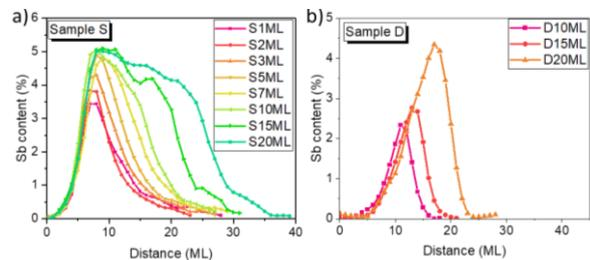
Fig. 2: Superposed composition profiles of Sb along the growth direction of samples S (a), and D (b) for different layer thicknesses.
