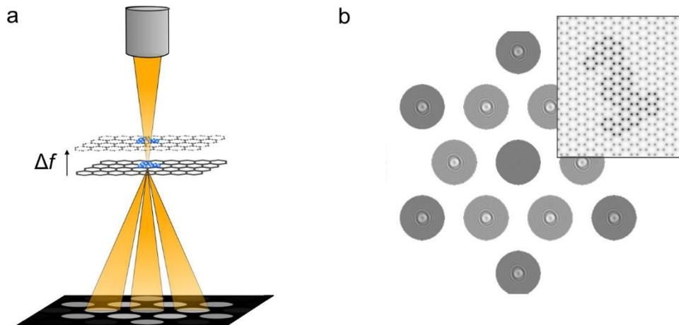
Fig. 1: (a) Sketch of the experimental scheme for CBED.  $\Delta f$  is the defocus. (b) Simulated CBED pattern of a carbon patch on top of graphene. Inset: The phase distribution of the transmission function.
