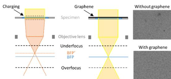
Fig. 1: Graphene-coated grids reduce charging and result in non-blurred images.
