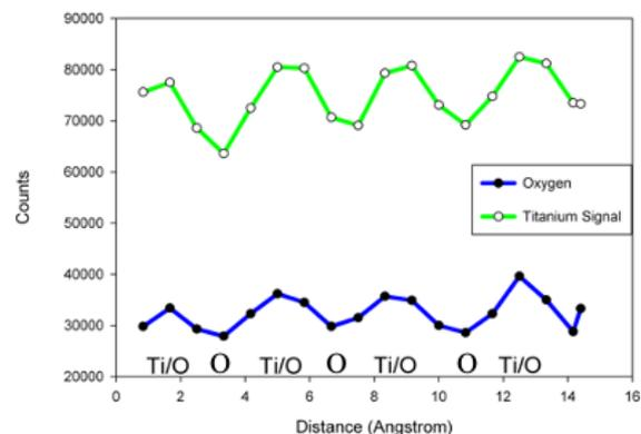
Fig. 1: EELS line scan from (001) STO monitoring the oxygen K-shell signal along successive Ti/O & O columns. The density of oxygen in both types of columns is identical but the O signal varies from column to column. [2]
