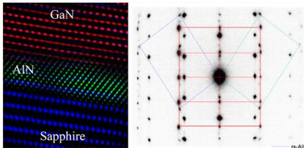
Fig. 1: Epitaxial GaN on sapphire with an AlN buffer layer
