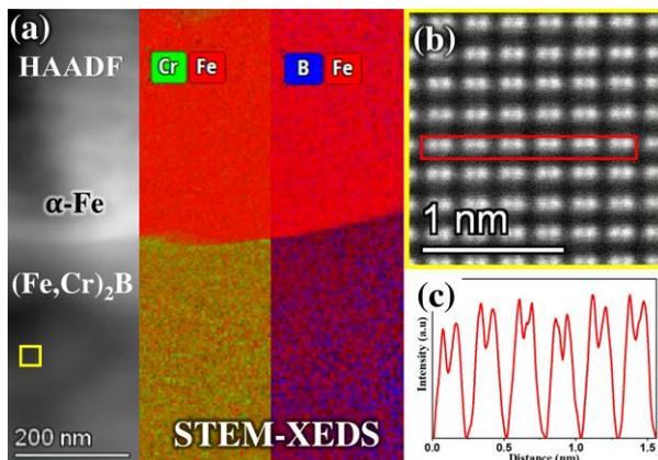
**Fig. 1:** (a) STEM-(HAADF+XEDS) of (Fe,Cr)<sub>2</sub>B and  $\alpha$ -Fe, (b) HAADF showing atomic arrangement with corresponding (c) atom column contrast in (Fe,Cr)<sub>2</sub>B.
