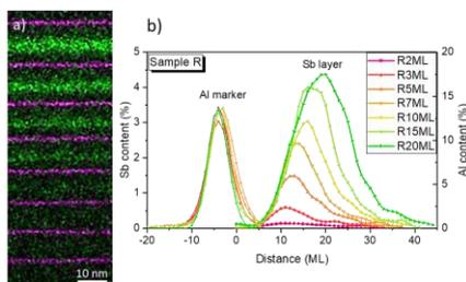
Fig. 1: a) EDX map of sample R showing Sb (green) and Al (purple) distribution. b) Composition profiles along the growth direction for different layer thicknesses.
