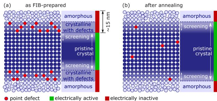
Fig. 2: FIB-induced structures of a lamella in the as-prepared (a) and healed state (b).
