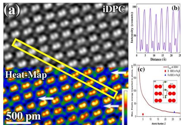
**Fig. 2:** (a) STEM-iDPC and heatmap showing inconsistencies in B atom position, (b) Intensity profile of (Fe,Cr) and B, (c) Energy imparted by 300 keV electron as  $f(z)$ .
