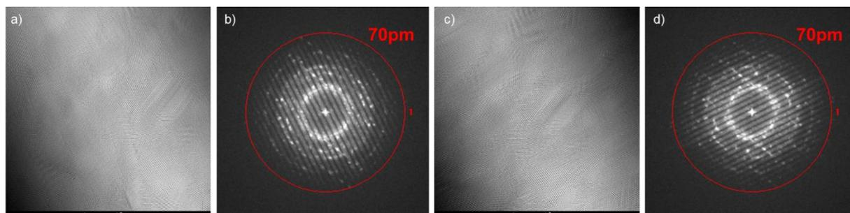
Figure 1: Information Limit of 80pm with 0.5mbar of N<sub>2</sub> in the octagon as determined by a young fringe experiment. a) displaced images in X, b) young fringes showing 70pm transfer in X, c) displacement image in Y, d) young fringes showing 80pm transfer in Y. These experiments show the atomic resolution capability in gaseous environment on the Spectra ETEM.
