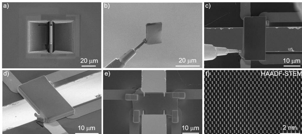
Fig. 1: Optimized FIB-based sample preparation workflow for in-situ electrical experiments. (a, b) Lamella extracted from bulk with alternative geometry. (c, d) Lamella in contact with E-chip. (e) Secure fixation to E-chip using Pt contacts. (f) HAADF-STEM image of thinned Si lamellae on E-chip.
