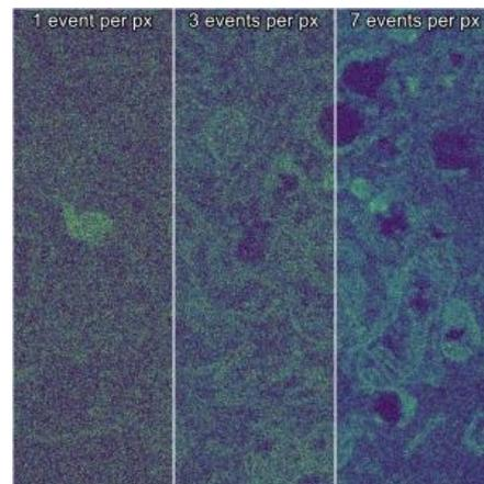
Fig. 2. Compositional image of human macrophage cells recorded with the beam blanker triggering after various event numbers per pixel.
