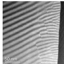
Fig. 2: A scanning moire fringe image showing defects in CdTe/ZnTe films grown on a GaAs substrate
