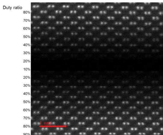
Fig. 1 HAADF image of Si [110] scanned using a pulsed beam.
