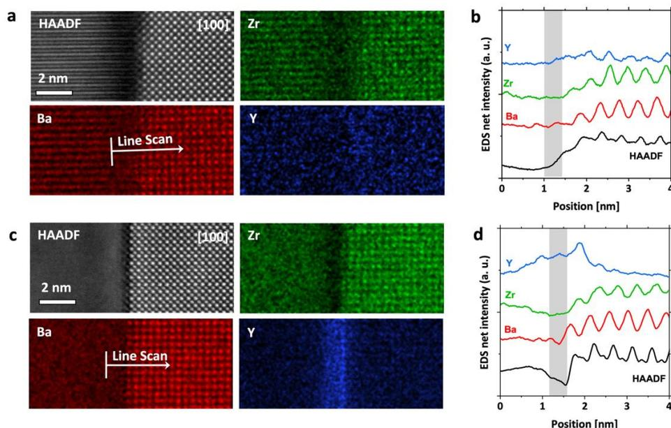
Fig. 1: HR-STEM EDS mappings of a non-equilibrium grain boundary without Y segregation (a, b) and a grain boundary after equilibration at 1600°C for 5h showing atomically sharp Y segregation.
