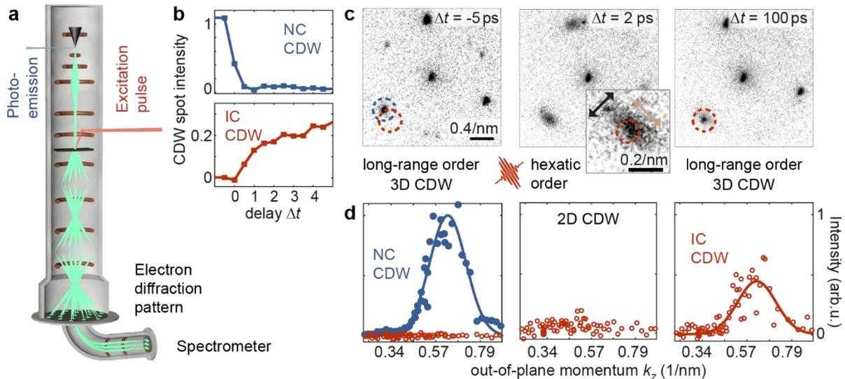
Fig. 1: **a** UTEM setup. **b** Suppression of the nearly commensurate (NC) CDW spot intensity (blue) after optical excitation and emergence of CDW spots characteristic of the IC phase (red). **c** Diffraction pattern at different temporal delays, showing the structural rotation of the NC to IC transition, and broadened spots indicative of a transient hexatic state. **d** CDW rocking curves acquired by beam tilting show the dimensional crossover into a transient 2D-state.
