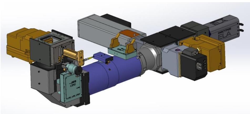
Fig. 1: Rendering of CEFID outfitted with five cameras (TVIPS XF416R, ASI Cheetah, Direct Electron DE-16 and Dectris ELA) and a retractable ADF detector developed by CEOS. Each detector has its specific strengths which make it ideal for a class of experiments.
