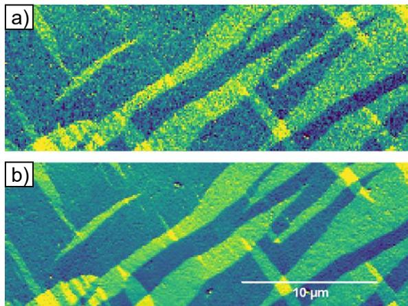
Fig. 1: STEM-DPC measured vertical deflection of probe from freestanding LSMO at a) close to a zone axis b) 7.5° tilted away.
