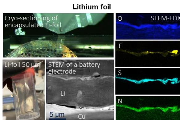
Fig. 2: Cryo-ultramicrotomy of lithium foil for battery solid electrolyte interphase research
