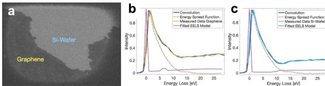
Fig. 1: a) BSE image of a graphene flake on Si-wafer. b) for graphene and c) for SiO<sub>2</sub> show the expected EEL spectra from known TEM measurements (purple, [2] and [3]) and a naïve model fit (convolution of TEM data with the energy spread function of the DELTA, blue).
