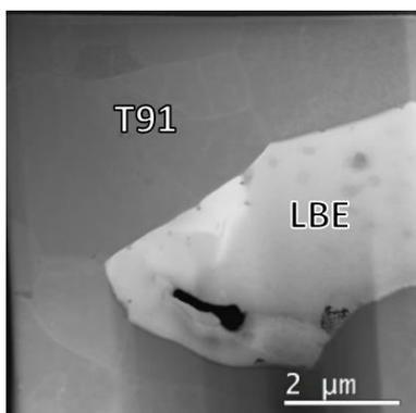
Fig. 1: STEM HAADF view of the TEM lift out foil of reducing environment corroded sample.
