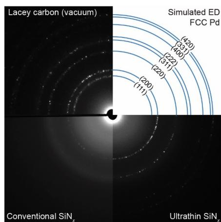
Fig. 2: Improvement of ultrathin membranes in diffraction analysis.
