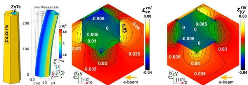
Fig. 2: Quasi tomographic reconstruction of lattice distortion tensor components  $\epsilon_{xx}$  and  $\epsilon_{yy}$  in NW cross-section maps of relative strain, calculated using relaxed ZnTe as a reference-best fit.
