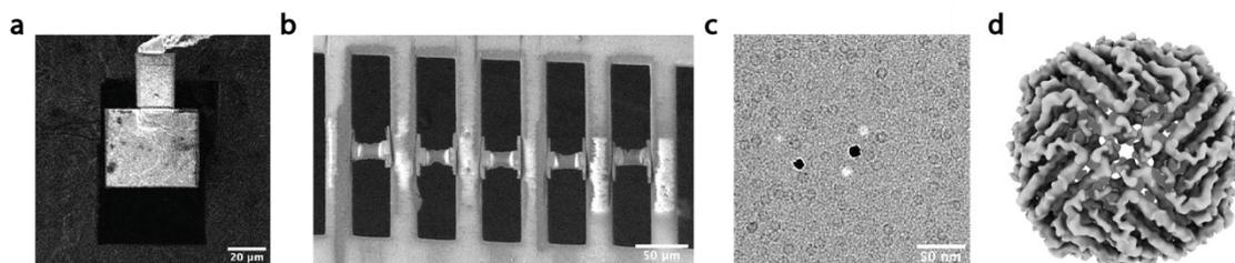
Fig. 1: Serial lift-out for high-resolution cryo-EM. (a) Ion beam image during lift-out of vitrified sample block from high-pressure frozen sample. (b) Scanning electron microscopy image of a series of polished lamellae after lift-out. (c) TEM image of high-pressure frozen and FIB-milled apoferritin sample, dark spots are Pt particles from sputter coating. (d) Apoferritin reconstruction at 5.8 Å from 1115 particles.
