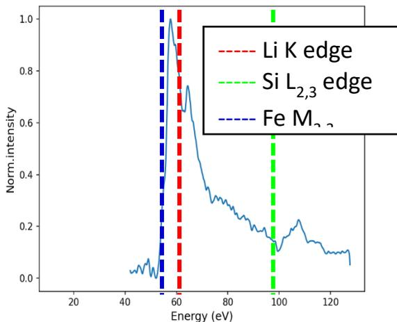
Fig. 1: EELS spectrum of  $\text{Li}_2\text{FeSiO}_4$  taken with the Hitachi SU-9000 at 30 keV.
