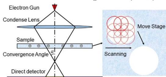
Fig. 1: Schematic diagrams of the optical configuration for ptychography
