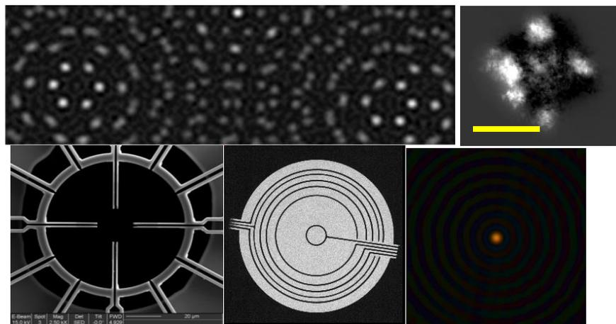
Fig. 2: Top: from left to right: Simulated CGI reconstruction of atomic resolution, experimental CGI with 1 nm resolution (scalebar is 20 nm). Bottom: MEMS design for CGI, for aberration correction and best expected probe in the order of 1 Å.
