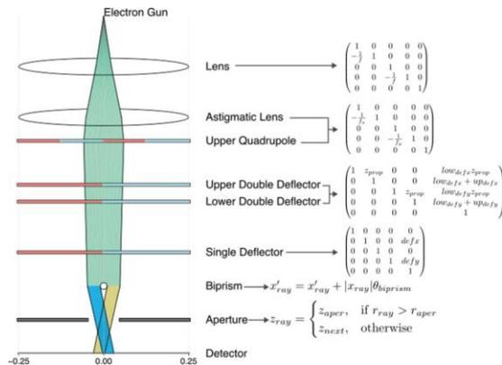
Fig. 1: Ray tracing simulation of a transmission electron microscope (TEM) [2].
