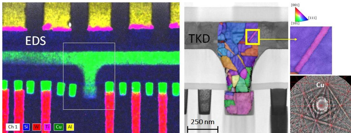
Fig. 1: Composition and crystallographic grain structure of a Cu interconnect studied at nm resolution. Note the intermixing of Si and Cu signals in EDS at the lower end of the connect.
