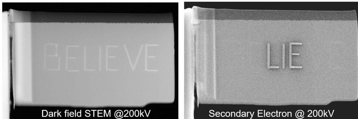
Figure 1: When surface information matters. Simultaneous SEM & STEM image of a TEM Lamella. The letters "LIE" are deposited on the front side and the letter "BE" and "VE" on the backside.
