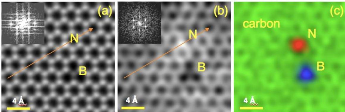
Fig. 1. a) MAADF image, b) SE image (Gaussian filtered), c) EELS elemental maps of the same area of graphene with B and N substitutions.  $E_0 = 60$  keV.
