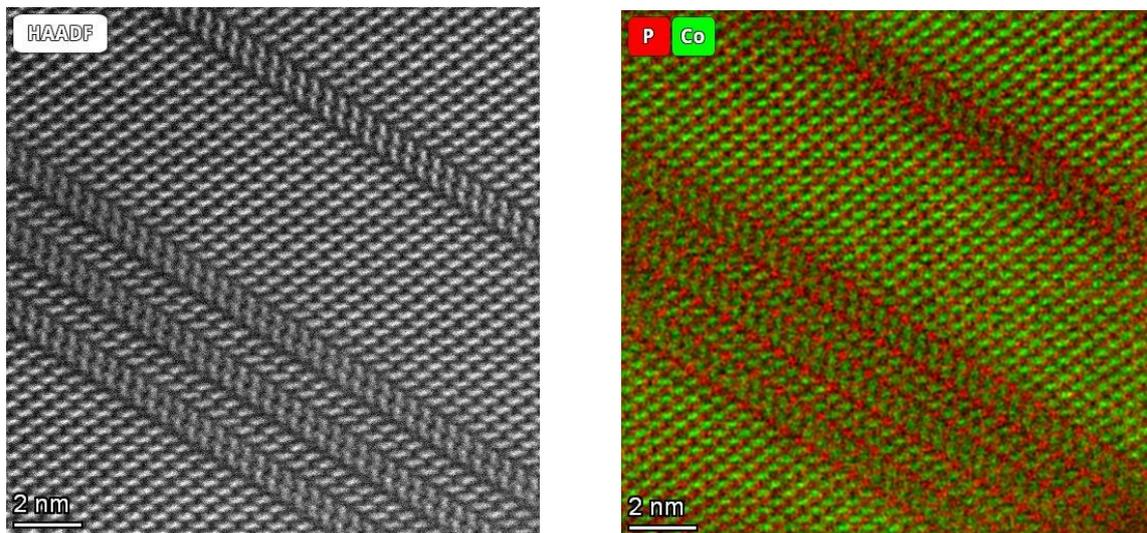
Fig. 1: Atomically resolved HAADF-STEM image of LiCoPO<sub>4</sub> cathode material alongside the corresponding Ultra X EDX map collected with a total dose of  $\sim 4000 \text{ ke}/\text{Å}^2$  at 300 kV accelerating voltage. Electron dose mitigation workflow was used prior to the EDX data collection.
