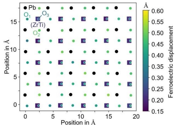
**Fig. 2:** Measured ferroelectric displacements in  $\text{PbZr}_{0.2}\text{Ti}_{0.8}\text{O}_3$  from experimental 4D-STEM data. The precision amounts to 3 pm.
