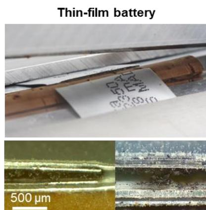
Fig. 1: Cross-sectional preparation of commercially available Li/MnO<sub>2</sub> thin-film battery by self-built cryo-cutter tool
