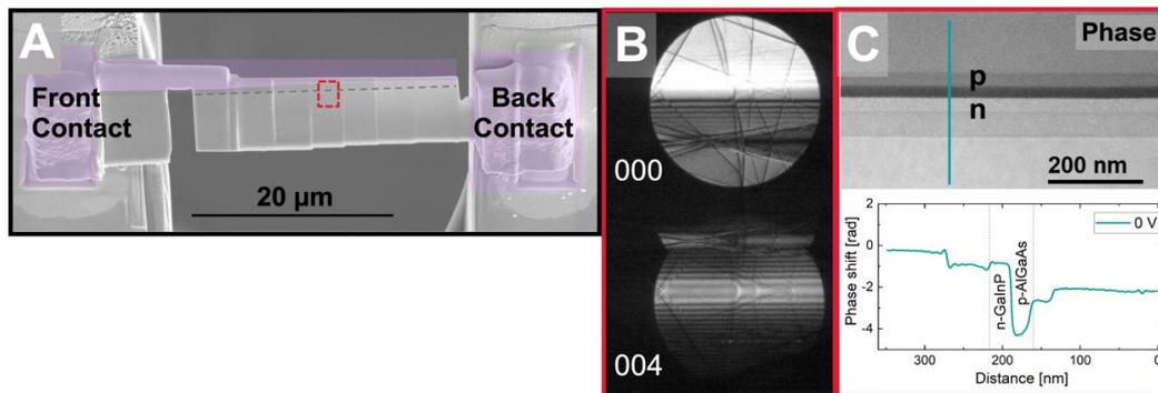
Fig. 1: A) Scanning electron microscope image of a TEM lamella with regions of different thickness prepared by FIB milling and mounted on a chip for *in situ* electrical biasing. B) STEM-CBED pattern recorded at the ROI indicated in A to derive the crystalline specimen thickness. C) Electron phase image reconstructed from an off-axis electron hologram stack recorded from the same ROI, and the corresponding line profile extracted from the phase image across the junction.
