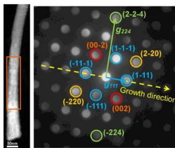
Fig. 1: Curved ZnTe/CdZnTe core-shell NWs, single NB diffraction pattern and FEM model of NW
