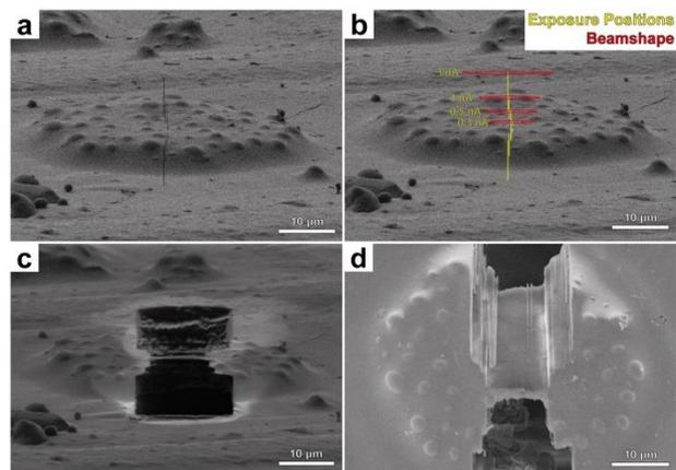
Fig. 2: Lamella milled using an ion knife. a) Cryo-FIB image of yeast cells prior to milling. b) Exposed positions with the shaped ion beam. Red ellipses indicate the beam shape. Yellow lines indicate the exposure positions. c) FIB and d) SEM image after lamella preparation.
