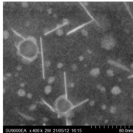
Fig. 2: Li EELS jump ratio map of an Al 2099 alloy taken with the Hitachi SU-9000 at 30 keV.
