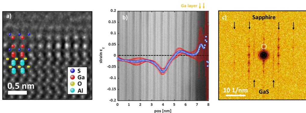
Figure 1: a) HR-STEM of the GaS monolayer sample showing the additional Ga ad layer.\* b) Strain  $\epsilon_z$  in the growth direction derived from GPA analysis and superimposed onto the HR-STEM image of the GaS multilayer sample. c) Combined FFTs of the sapphire substrate and the GaS adlayer showing the in-plane relaxation.
