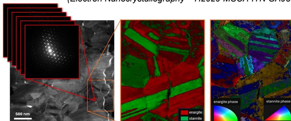
Fig. 1: (Left) STEM image of the  $\text{Cu}_{2.3}\text{Mn}_{0.7}\text{GeS}_4$  [2] nanocomposite made of enargite and stannite phases. Precession-assisted 4D-STEM was used to obtain both 3D ED type data for crystallographic structure analysis (in red) and phase (middle) and orientation (right) maps from the same ROI (orange rectangle).
