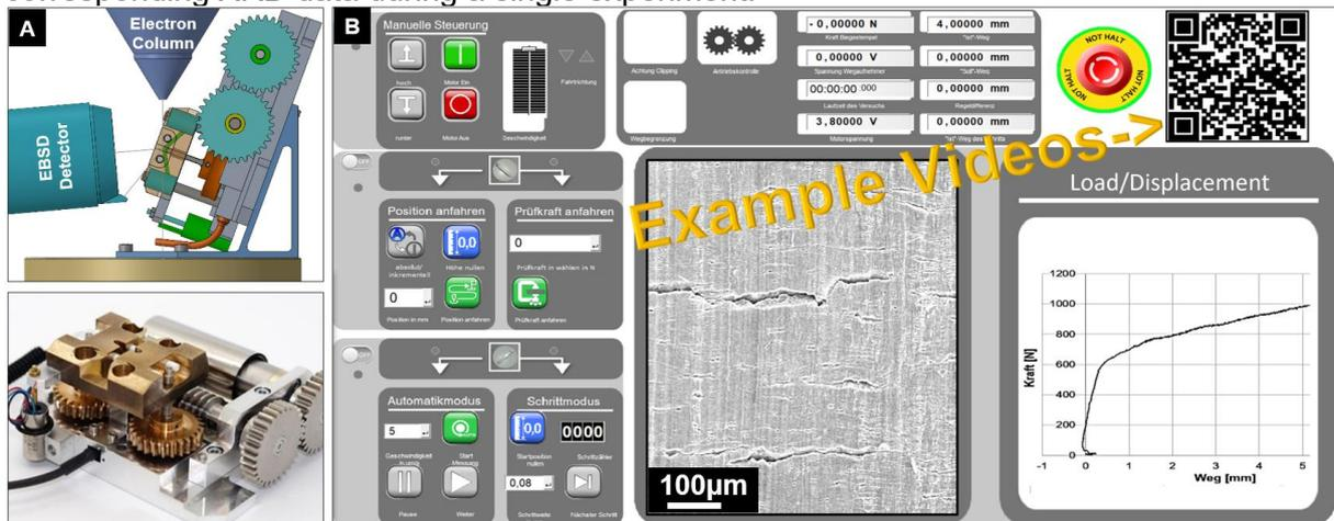
Fig. 1: A (top) CAD model of the miniaturized 3-point bending machine, (bottom) complete set-up after development, B) Graphical User Interface showing exemplary measurement in progress
