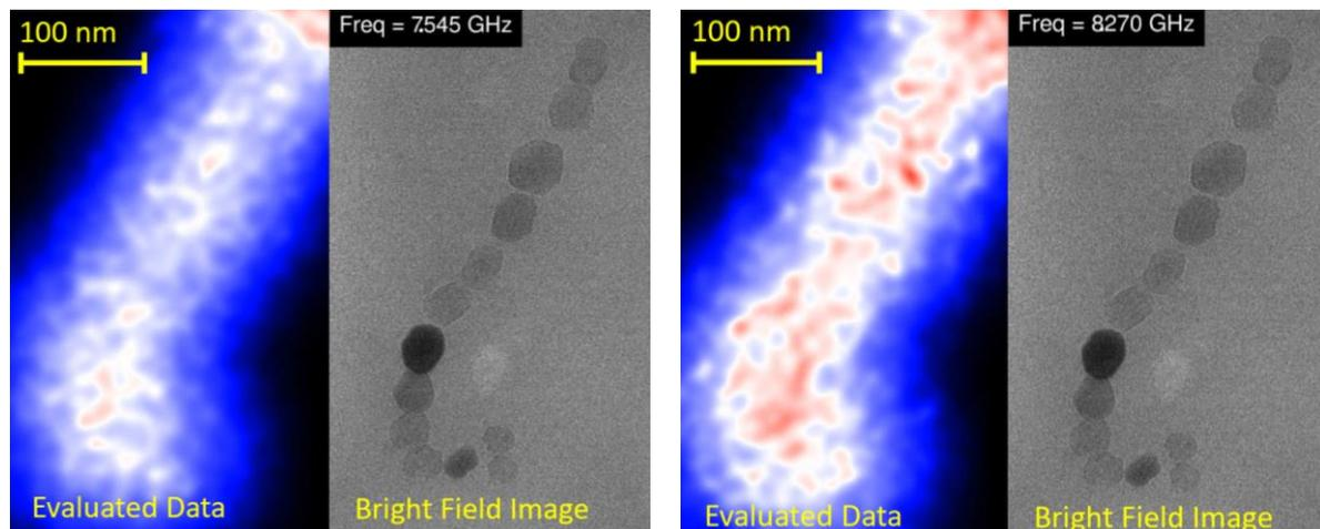
Fig. 1: Spin wave amplitude distribution off resonance (left) and bright field image (right). Fig. 2: Spin wave amplitude distribution in resonance (left) and bright field image (right).
