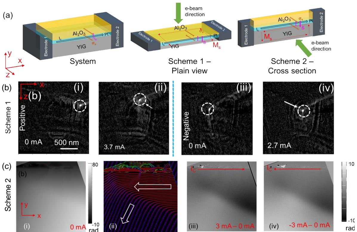
Figure 1. (a) Different schemes of YIG/Pt used for the study, (b) switching of magnetic vortex using spin currents and (c) domain wall oscillations observed in electron holography.
