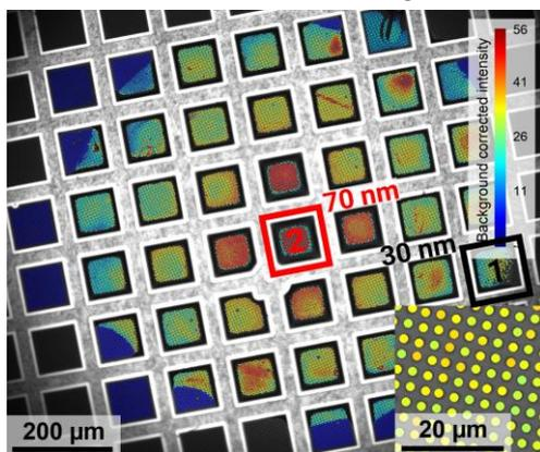
Fig. 1: VitroJet deposition image with intensity color overlay, which correlates with ice thickness
