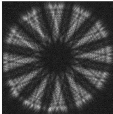
Fig. 1: Interference pattern generated with an AdaptEM 16 element programmable phase plate for electrons, showing the ability to adjust the wavefront of a coherent electron wave as a new degree of freedom in electron microscopy.
