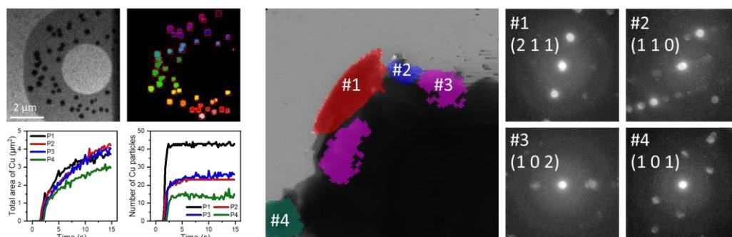
Fig. 1 Data processing of in-situ TEM. (a) Tracking size and number of Cu particles during electrodeposition. (b) Orientation analysis of electrodeposited Zn via 4D STEM analysis
