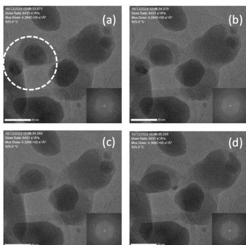
Fig. 1: The evolution of two Au NPs sintering (a-d) highlighted in the dashed circle.
