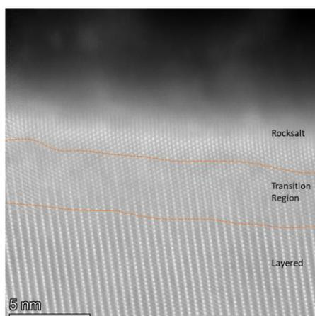
Fig. 1: HR-STEM image of layered Ni-rich NMC with reconstructed surface layer.
