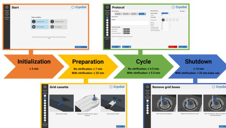
Fig. 2: VitroJet workflow to automatically prepare high quality samples for high-throughput cryo-EM.
