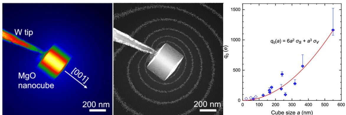
Figure (Left) Phase map of a MgO nanocube with a size of 260 nm acquired at a dose rate of  $4.1 \text{ e}\text{\AA}^{-2}\text{s}^{-1}$ . (Middle) Corresponding phase contours with a contour spacing of  $2\pi/8$ . The electron beam direction is close to the  $\langle 110 \rangle$  zone axis. (Right) Charge vs. size of the MgO nanocubes. The parabolic dependence suggests that the charge is mostly localized on the surfaces of the nanocubes.
