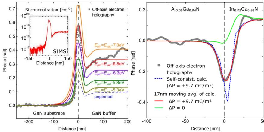
Figure (Left) Average profile of the phase change (gray symbols) across a  $\delta$ -doped GaN layer measured by off-axis electron holography. The lines represent self-consistent calculations of the phase change for different surface Fermi level pinning energies. (Right) This enables a calibration for subsequent measurements and analysis.
