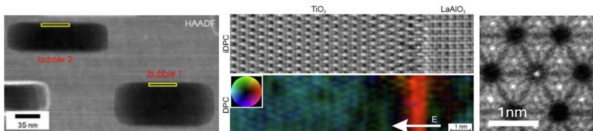
Fig. 1: (left) He bubbles within neutron irradiated beryllium. (middle) 2D electron gas at the  $\text{TiO}_2/\text{LAO}$  interface. (right) Cs atoms in the channel of beryl.
