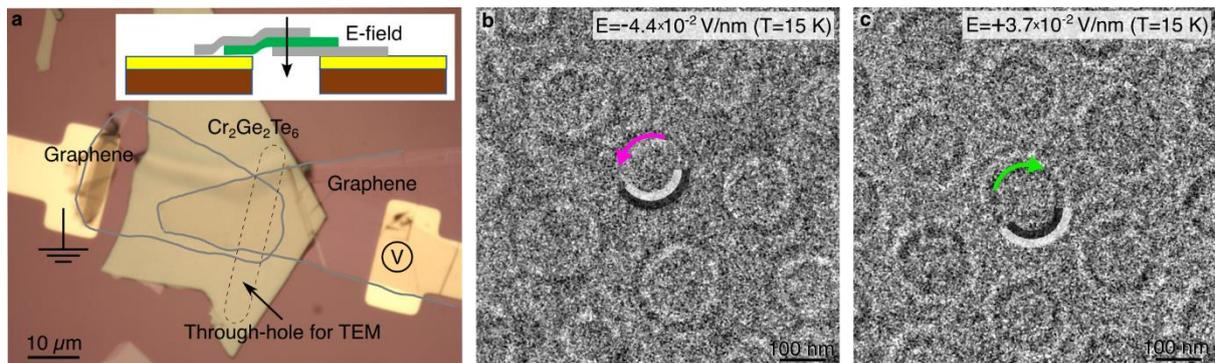
Figure 1: (a) Optical microscopy image of an electrically contacted graphene/ $\text{Cr}_2\text{Ge}_2\text{Te}_6$ /graphene heterostructure on a silicon/silicon nitride TEM grid with Pt electrodes. (b, c) Lorentz TEM images of the sample shown in (a) obtained at 15 K after field cooling in a magnetic field of 52 mT and with an applied electric field of (a) -44 mV/nm and (b) +37 mV/nm applied during field cooling.
