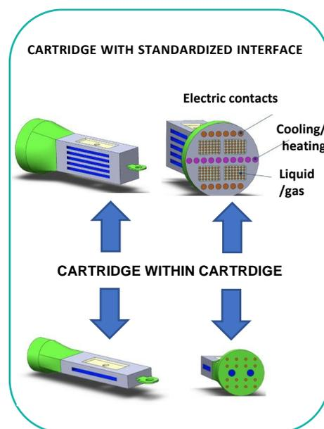
Fig 2. Schematic illustration of the proposed development in IMPRESS of cartridge in cartridge concepts and standardized interface that are compatible with larger numbers of electrical contacts, gases, liquids and light and can be inserted in different positions on a TEM column.
