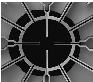
Fig. 1: Electron beam modulator, detail of the aperture
