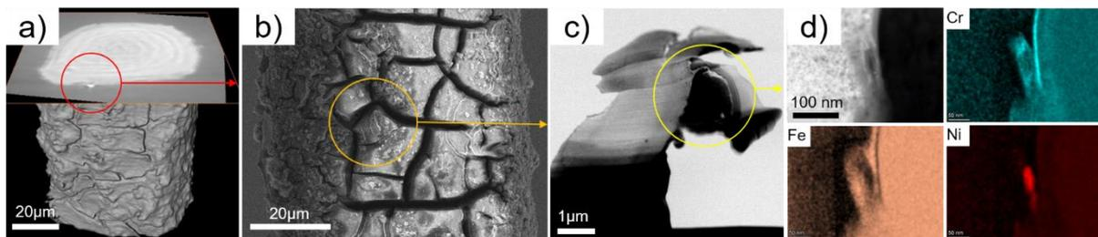
Figure 1: Correlative workflow: (a) SRnanoCT identification of ROI with impurity particle, (b) ROI identification in dual-beam FIB-SEM, (c) FIB lamella preparation within ROI, and (d) (S)TEM-EDX analysis at the particle-degradation layer interface.
