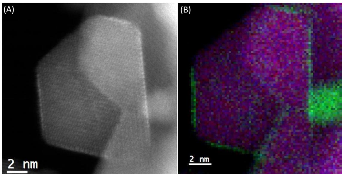
Fig. 1: STEM-EELS analysis of Ce-coated  $\text{Co}_2\text{O}_3$  nanoparticles (NPs). (A) Aberration corrected HAADF-STEM of Ce coated  $\text{Co}_2\text{O}_3$  NPs. (B) RGB composite of Co (red), Ce (green), and O (blue) showing one-atom thick layer of Ce atoms was found to covering a  $\text{Co}_2\text{O}_3$  NP.
