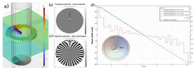
Fig. 3 a) optimal potentials and phase shift for a spiral phase plate b&c) phase before and after optimisation. d) optimal potential on boundary electrodes (red) and aimed phase shift (green and blue).
