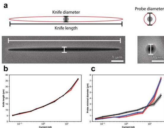
Fig. 1: Characterization of ion knife beam shapes. a) Definitions of the probe diameters and knife diameters and length for analysis. b-c) Measurements of b) knife length and c) minimal knife diameter for different currents.
