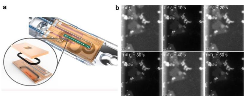
Figure: Time series of *in situ* STEM images in a LPTEM holder (a) showing the repeatable removing and refill of liquid by purging with an inlet gas pressure of 3 bar.
