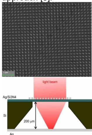
Fig. 1: Metalens system to increase numerical aperture and produce localized electron beam shaping
