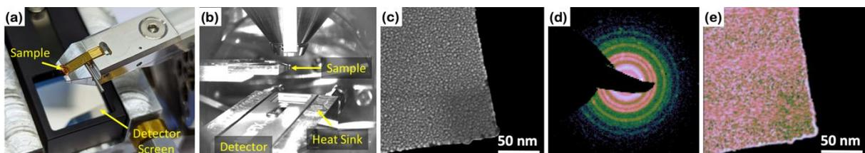
Fig. 1. (a) Sample holder and detector assembly, (b) In-chamber situation of Zeiss Merlin® during 4DSTEM data collection, (c) SEM image of Pt thin film with nano grains, (d) 4D data set using data processing algorithms, and (e) virtual DF image.
